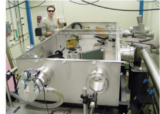
Existing HERCULES 500 TW compressor
