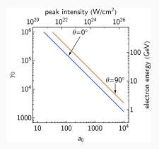
$\gamma_0 = \text{initial electron energy}$  $a_0 = \text{peak laser intensity}$ duration =  $50\lambda$  ? Can we reach  $\alpha \chi^{2/3} \sim 0.1$ ? (10% loop corrections)
