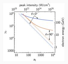
$\gamma_0 =$  initial electron energy  $a_0 =$  peak laser intensity duration  $= 50\lambda$
